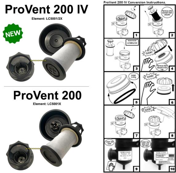
WARNING: Only install LC5001/2X after conversion completed.
